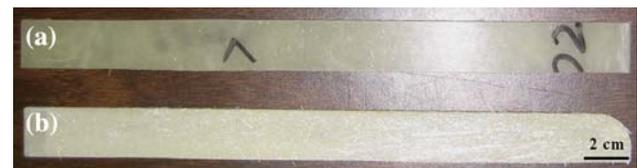
**Fig. 2** (a) Unexposed beam and (b) UV exposed beam. Damage caused by UV can be seen in the form of many fibers exposed at the surface
