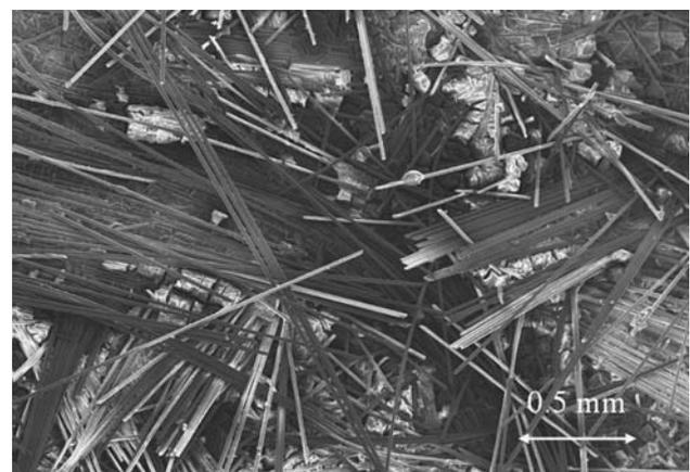
**Fig. 8** LFT exposed for 1,600 h to UV radiation. Most of the matrix in the surface region has disappeared and exposed fibers can be seen
